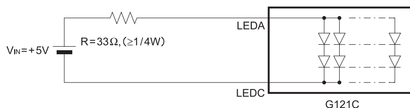
Figure 14 LED Backlight Driver Example 1
