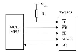
Figure 3. Use of Pullup Resistor on /CE
