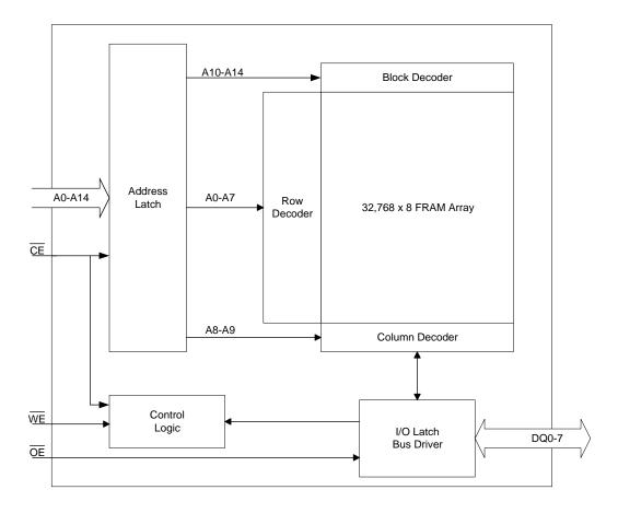
Figure 1. Block Diagram
