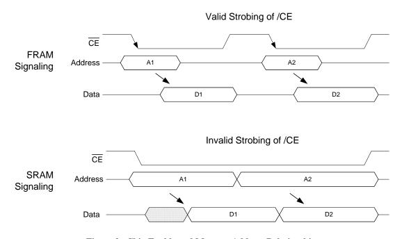
Figure 2. Chip Enable and Memory Address Relationships
