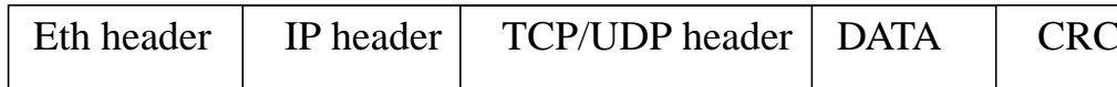
Figure 5.3: One Ethernet frame encapsulate the IP packets. Each layer includes a header and data.
