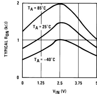
FIGURE 7. Multiplexer  $R_{ON}$  vs  $V_{IN}$
