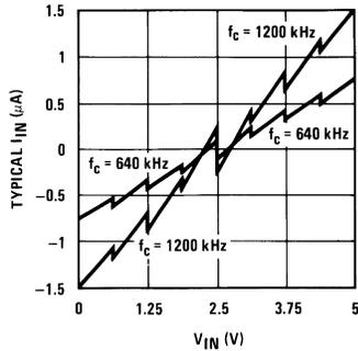
FIGURE 6. Comparator  $I_{IN}$  vs  $V_{IN}$
