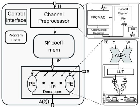
Fig. 4: Block Diagram of the Dual-mode MIMO Detector
