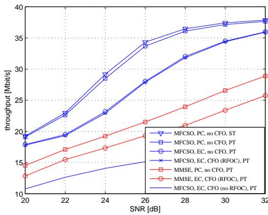
Fig. 7: Coded Throughput ( $2 \times 2$  SM, CQI=15, 5 MHz band)
