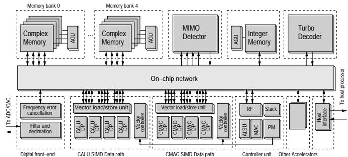
Fig. 3: Baseband Processor Architecture Overview
