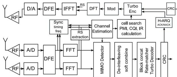
Fig. 1: Functional Flow of an LTE Modem (PHY only)
