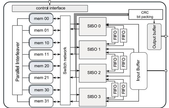
Fig. 5: Block Diagram of the Parallel Turbo Decoder
